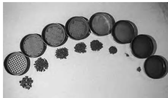
Figure 25.3 – Aggregate Combined Grading determined by Sieving
