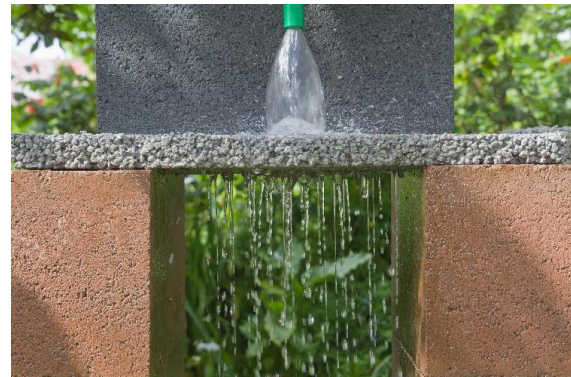
Figures 24.1 – A Permeable Paver Demonstration, Austin's Ferry, Tasmania, Australia 24.1
