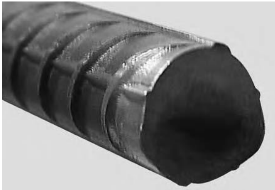
Figure I.19 – Typical 500-MPa Deformed Bar
