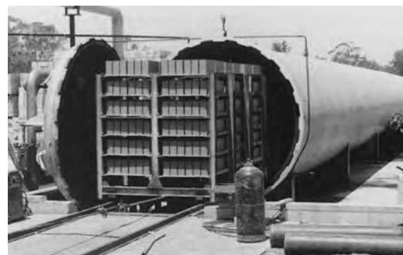
Figure 15.11 – Autoclave Equipment used to Harden and Cure Concrete Blocks
