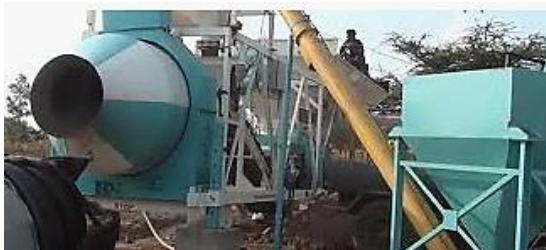
Figure 9.4 – Typical Small On-site Plant with Capacity of about 10 m 3 per hour.
