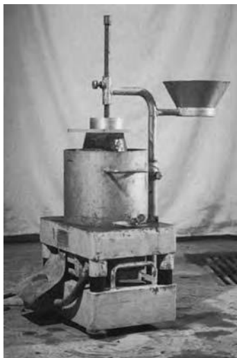
Figure 25.7 – The Vebe Test
