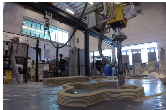
Figure 24.7 – Robotics and 3-D Printing, Extrusion-based Technique 24.7
