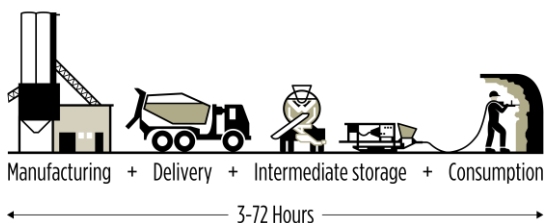
Figure 5.14 – HCA Used to Extend Working Time
