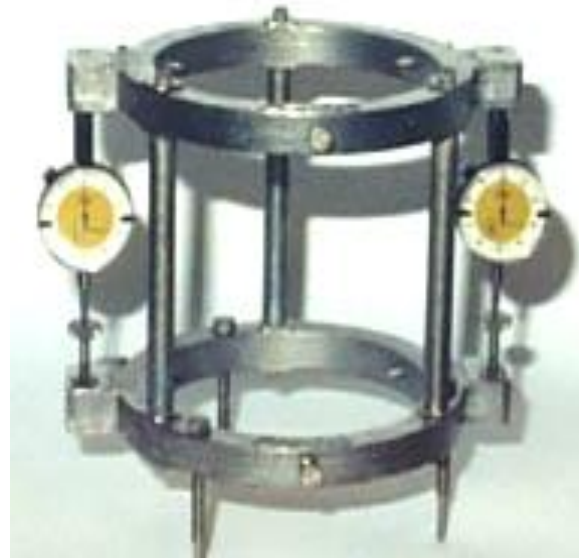
Figure 26.15 – Test Rig for Modulus of Elasticity
